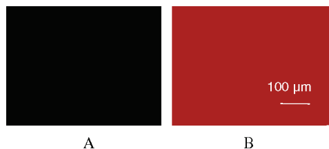
Figure 5. Homeotropically aligned optical textures of 2 at room temperature in a 2 \mu\text{m} thick cell: (A) with crossed polarizers; (B) without crossed polarizers; the textures are thermally stable from about 100 ^{\circ}\text{C} through room temperature.
